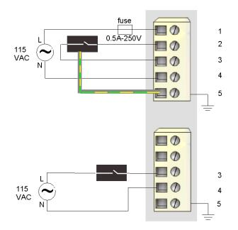
Within each connector, pins 1 and 2 are internally tied. The sensor on the top connector has a PE connection that is tied to the PE connection on the PDM base through pin 5.
