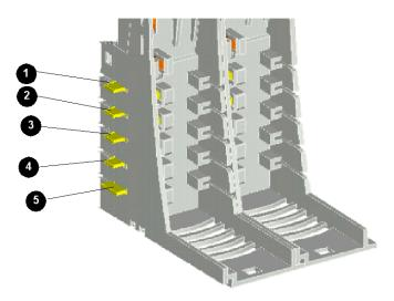
Field power (sensor power for inputs and actuator power for outputs) is distributed across the island bus to the STB XBA 3000 bases by a PDM:
