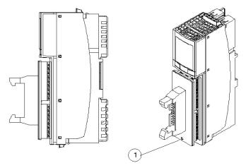
1 Make sure that this hole is positioned at the bottom of the module.
