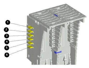
In the primary segment of the island bus, the signals that make these contacts come from the NIM. In extension segments, these signals come from an STB XBE 1000 BOS extension module:
