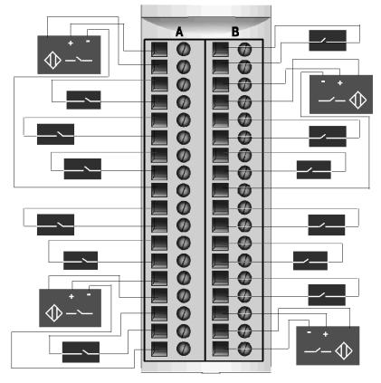
The following illustration shows you how you could connect four 3-wire sensors - one per input group - using the pins 9 and 18:
